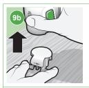
9b. Slowly pull the serter straight up without holding the buttons. Do not detach the pedestal from the serter in midair, as this might damage the sensor.
