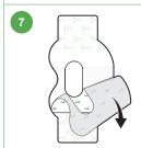
**7.** To apply a 2nd tape, remove liner 1.
