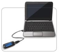
You cannot do a blood glucose test while the battery is charging. When charging is finished, the test strip port light will turn off. Unplug your CONTOUR NEXT LINK meter to test.
