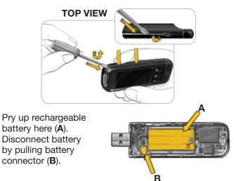
Dispose of the meter and lithium polymer battery in accordance with your local/country laws and regulations.
