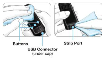
**2.** Dry all meter surfaces and test strip port using a clean paper towel if needed.
