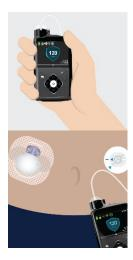
We call this technology SmartGuard<sup>™</sup> Auto Mode because it automatically adjusts insulin delivery. Since insulin is adjusted based on sensor glucose levels, a person must wear a continuous glucose monitor (CGM).
